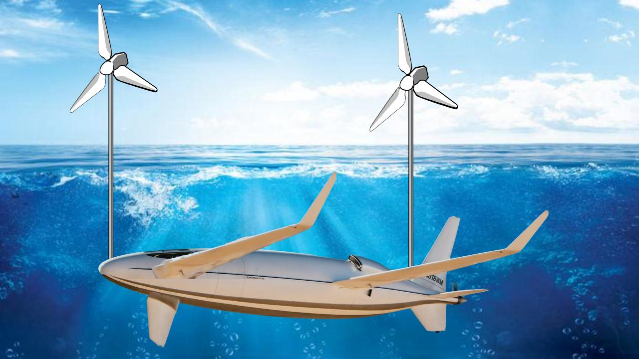
The idea of the invention is very simple. On the hull of a traditional modified submarine, as it resembles the fuselage of a commercial aircraft witha length of, for example, one hundred meters, two support poles for offshore wind turbine are mounted. Said turbines are mounted at the ends of the hull so that the blades of the two rotors do not interfere with each other.
